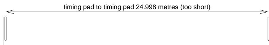
3) The upper tolerance on pool lengths is problematic when moveable bulkheads are installed, especially when more than one has been incorporated. It also causes difficulties when timing pads of a thickness other than that used for the design are supplied.
