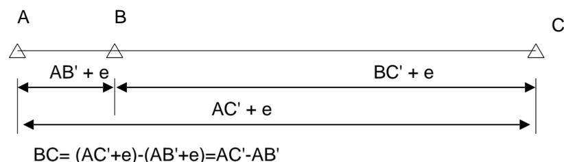
Note that apparently identical targets and reflector surfaces can have different constants. It is not unusual to find a spread of 2 millimetres across a batch of, say, 10 prisms. Ideally the pre-survey checks should use a single prism and this prism should then be used for all subsequent measurements.
